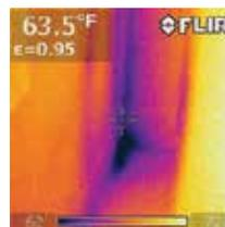
**Infrared thermographic surveys are used to find abnormal thermal patterns or temperature differentials that may reveal moisture leaks that could lead to mold growth.**
